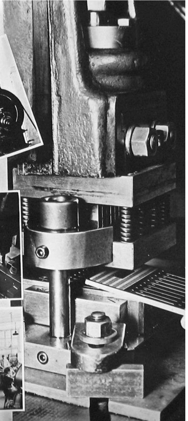
Schlitzen der Kassetten slotting of etched metal casing
